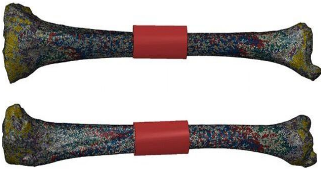
Figure 1: Finite element model of the tibia with a biomaterial colored in red implanted in a large diaphyseal lesion. Views of the model in front (a) and sagittal (b) plane.
