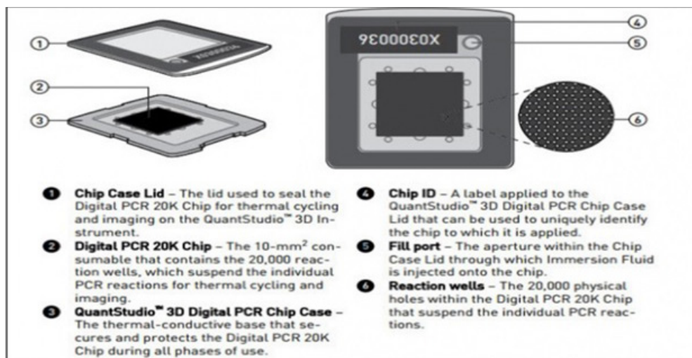
Figure 2: Diagram illustrating Quant Studio™ 3D Digital PCR System Chip; ChipCase Lid (1); Digital PCR 20 K 10 mm 2 nanofluidic v2 chip case and lid (2), which contains 20,000 reaction wells; QuantStudio™ 3D Digital PCR Chip Case (3); Chip ID (4); Fill port (5); and Reaction wells, the 20,000 physical holes (6) that suspend individual PCR reactions. Modified from reference 167.
