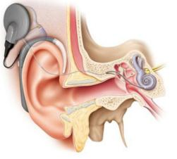
Figure 1: Representation of a cochlear implant, from the receptor, speech processor and the electrodes
