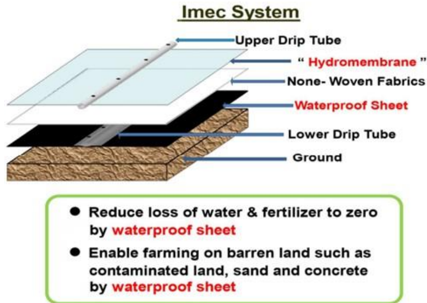
Figure 2: The Construction of Imec System.
