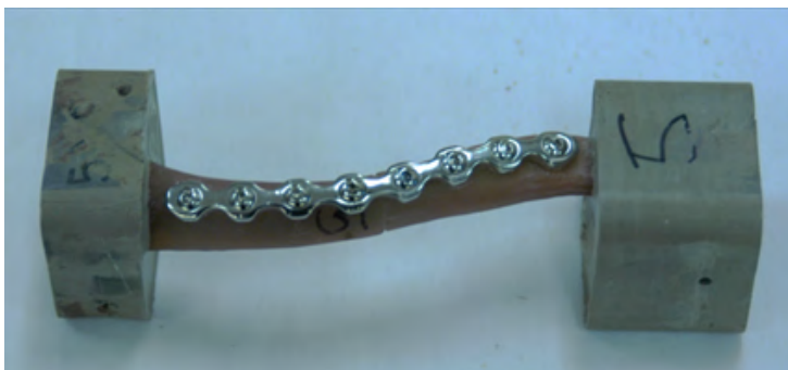
Figure A2. Sawbones 4th generation composite clavicle with manufactured mid-shaft osteotomy repaired using contoured Synthes eight-hole 2nd generation 3.5mm locking pelvic reconstruction plate on the superior surface.
